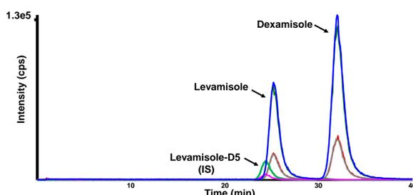
**Fig.2:** Chiral LC-MS/MS chromatogram of levamisole/dexamisole and the internal standard (IS) levamisole-D5; analyte separation on a chiral AGP column (100 mm x 4 mm, 5 μm).
